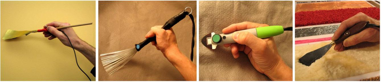
Figure 2. The four wands that were created for *The Sound of Touch*. From left to right they are the Brass Blade (too flimsy), the Drum Brush (good for uniform textures, but everything sounds similar), the Plastic Wand (good control, but absorbs too much vibration) and the Painting Knife (best).
